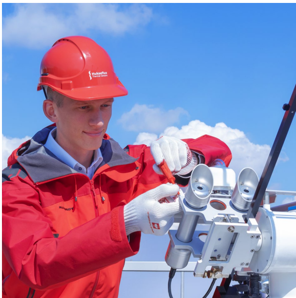
Figure 2 The importance of heating: tracker-mounted operation of heated DR15-A1 and DR20-A1 pyrheliometers, here being installed with heated SR15-A1 pyranometers. The data availability of non-heated instruments suffers in almost all environments due to morning dew and frost.
