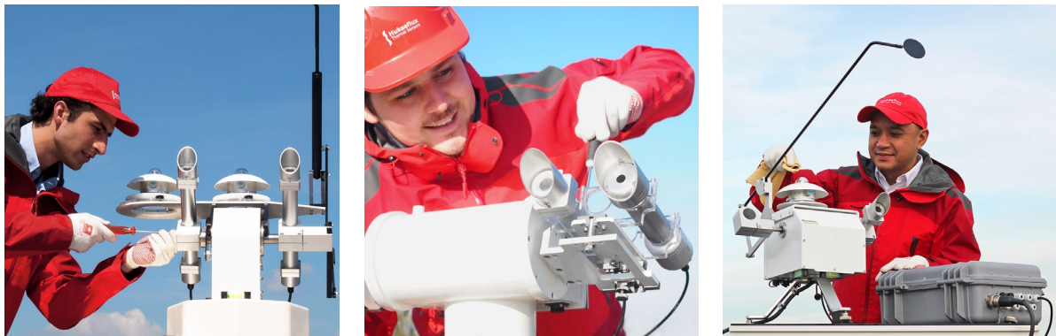
Figure 0.4 Applications of DR30 and other pyrheliometers, mostly combined with pyranometers, in typical solar radiation monitoring stations.
