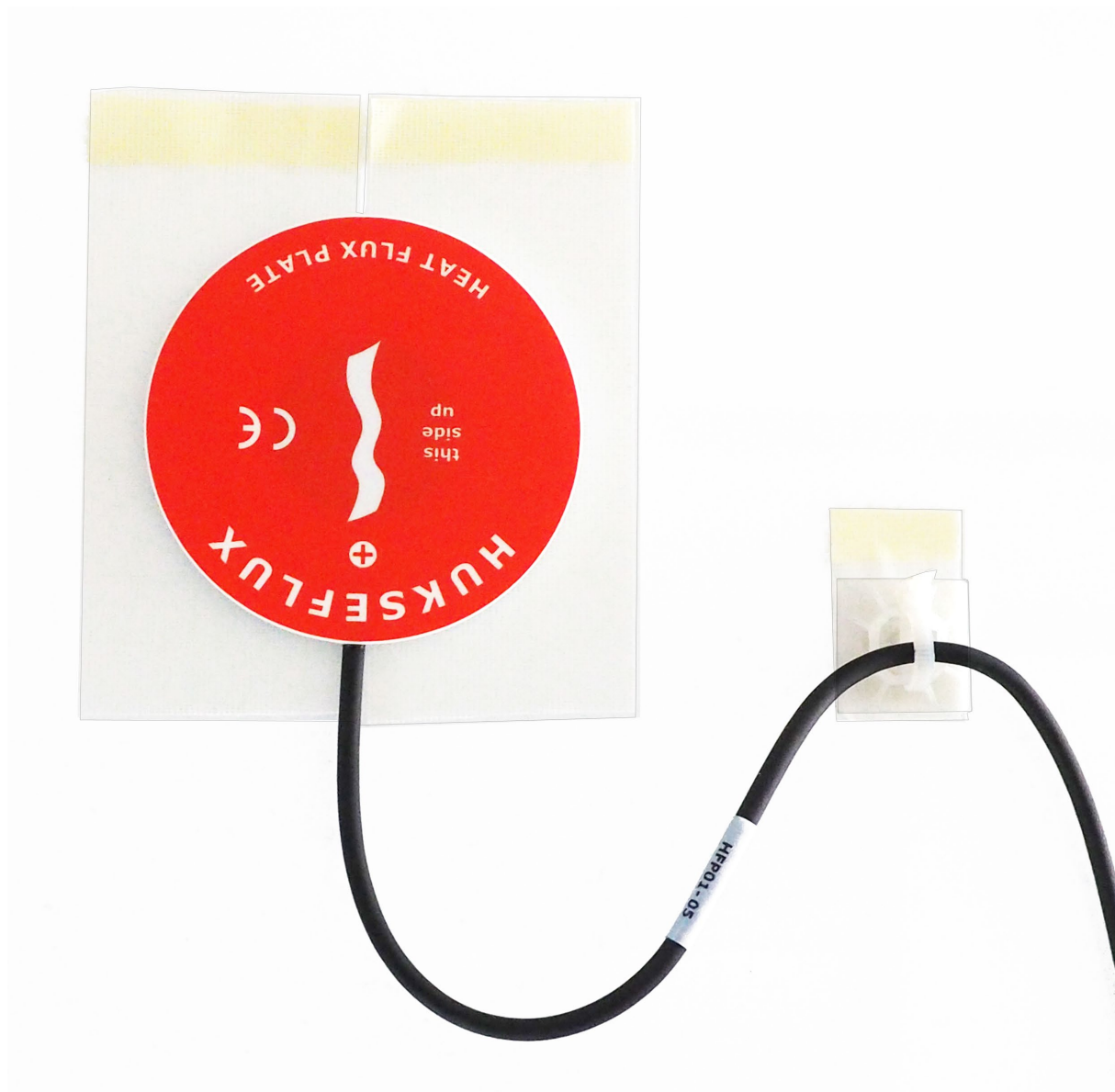
Figure 5.1.1 Installation of HFP01 on a wall using sided "removable" carpet laying tape such as TESA 4939, and a strain relief of the cable using a cable tie mount equipped with the same carpet laying tape as adhesive.
