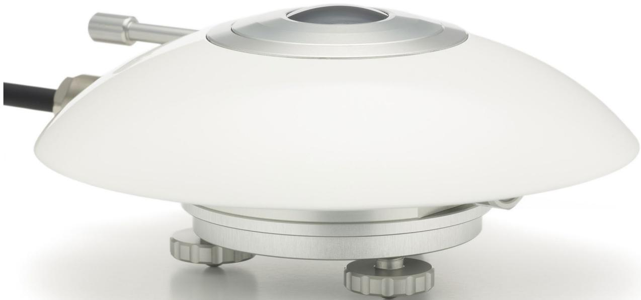
**Figure 1** IR20 research grade pyrometer.
