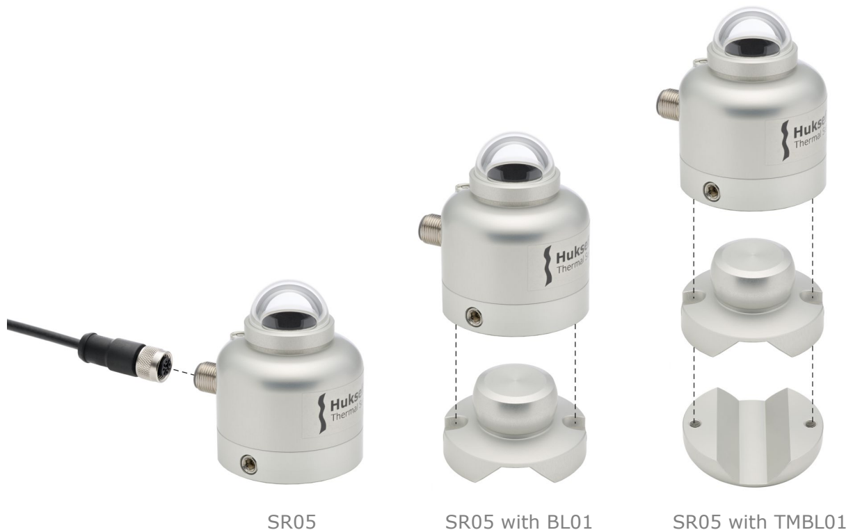
Figure 5.2.1 From left to right: SR05 in its standard configuration with 3 metre cable; with optional ball levelling for easy mounting and levelling on a (non-)horizontal surface; with optional ball levelling and tube mount for easy installation on a 25 to 40 mm diameter tube. Mounting screws are included with the ball levelling and / or tube mount.
